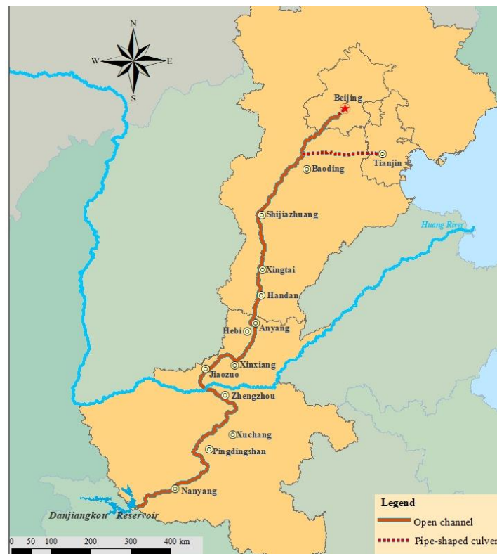
Figure 1. Middle Route of the south-to-north water diversion project.
